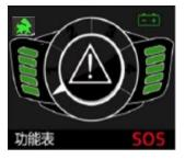
Communication failure: The wheelchair cannot drive. Communication system is broken. The center icon is the exclamation mark.
