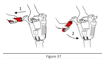
Release the secure lever of the back handle (1) and bring the handle to 100 degrees position (2). Allow the seat to slide down until it clicks in place (3). (See Figures 38 and 39).
