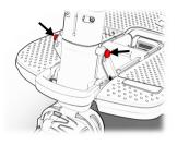
Figure 26 Steering Rod angle adjustment screws
