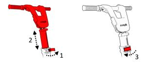
Figure 22 Driving Console height lever
