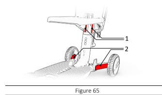
All the bearings on your ATTO are permanently lubricated and sealed and therefore no lubrication is required.
