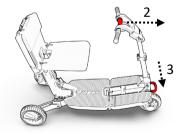
10. Place one hand on the tiller and with the other hand release the secure lever of the back handle (1), bring the handle to an upright position of 90 degrees (2) (see Figure 13).
