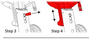
Figure 25 Seat height adjustment holes
