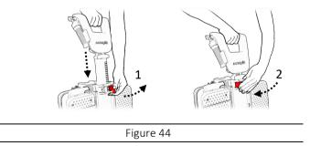
Release the adjustment lever of the handlebar (1) and bring the handlebar to a horizontal position (2). Then bring the lever back to secure position (3). (see Figure 45).
