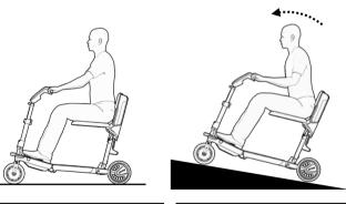
Figure 35 Normal driving position Figure 36 Shifts center of gravity
