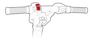
Figure 31 Reverse and horn buttons
