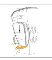
Pull to open zipper slider to ensure battery space filler is free (don't forget to remove your ATTO battery)
