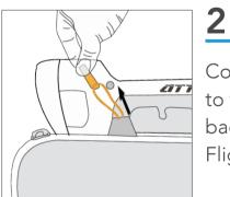
Connect the two loops to the hooks on the backrest to ensure Flight Kit positioning
