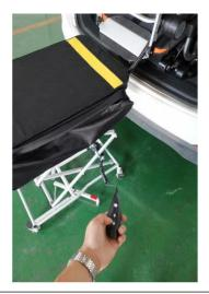
A14. Keep pressing the Down button on the controller, so that the platform is totally closed.
