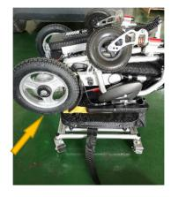
A4. The wheelchair is placed on the tabletope in an inverted direction as shown in the picture with the wheels in contact with the edge of the tabletop.
