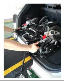
A12. Manually grasp the position in the picture to lift the wheelchair.
