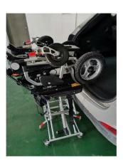
B8. The tyres are in contact with the edge of the tabletop as shown in the picture, to ensure that the wheelchair is stably placed.
