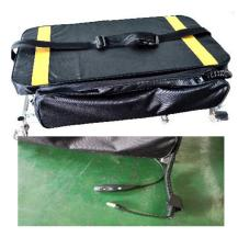
B1. Take out the controller and power plug from the battery pack
