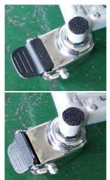
B6. Step on the brakes on four castors, and ensure that the wheel cannot turn
