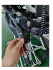
A10. Place the controller into the battery pack to prevent any damage.
