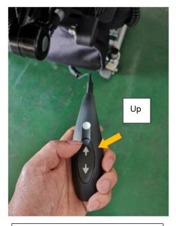
A6. Keep pressing the Up button on the controller, till the tabletop reaches the bottom surface of the trunk of the vehicle.
