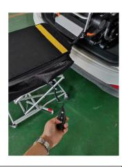
B4. Keep pressing the Up button on the controller, till the tabletop reaches the bottom surface of the trunk of the vehicle.
