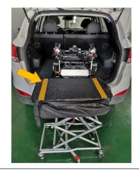
A13. Push it into the trunk, and guarantee that the wheelchair is stably placed. Release the brakes on all castors
