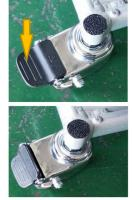
A2. Step on the brakes on four castors, and ensure that the wheel cannot turn
