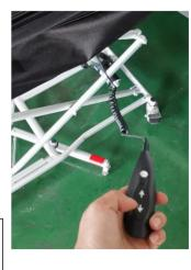
B11. Move the platform car from the vehicle, and ensure that the platform car will not collide with the vehicle during the lowering operation. Keep pressing the Down button on the controller, so that the platform is totally closed.
