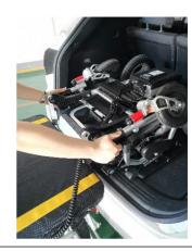
B7. Manually grasp the position in the picture to lift the wheelchair. Move the wheelchair from the trunk to the platform car
